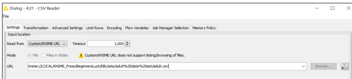
Figure 2.15. Automatic configuration of the Input Location part in the Settings tab of a CSV Reader node created via drag & drop of a file from the KNIME Explorer panel into the workflow editor panel.
