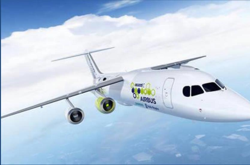
The BAe 146 demo aircraft will at first have one of its four engines replaced with an electric engine, powered by batteries and an onboard generator using jet fuel. The team will then move to two electric engines once the technology is stable.
